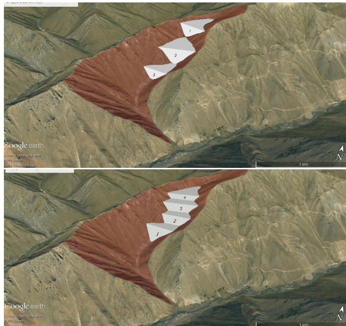
Figure 7: Options for the placement of the dump according to the calculations of numerical modeling of the slope and the overburden dump.
